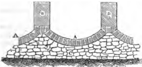
Fig. 28—Section of vertical supports on reversed arches. A, reversed arch. B, vertical supports. C, bed of stone.
